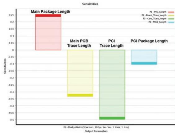
▲ DOE results for several significant parameters in PCI Express interconnect simulations. The PCI trace length on the peripheral card had the greatest negative impact on the eye opening, followed by the main PCB trace length.
