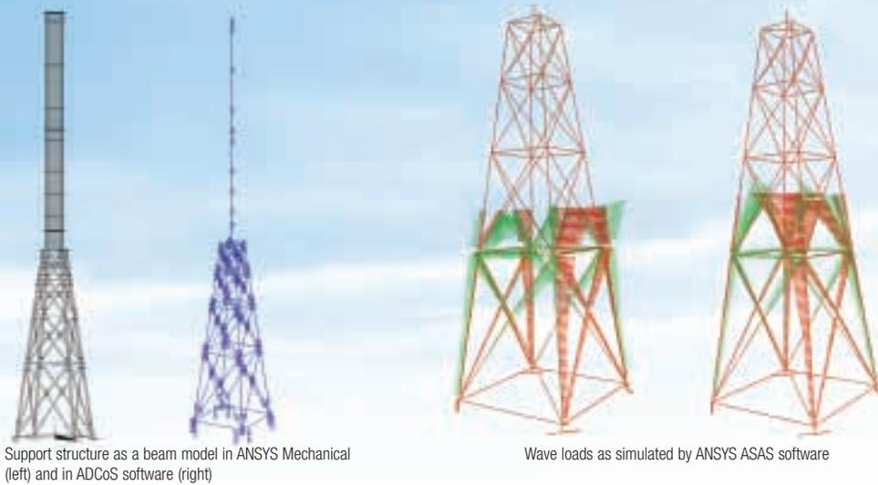
ASAS-WAVE to calculate the wave loads on the support structure. With the aid of ASAS-WAVE, loads resulting from linear and nonlinear waves, as well as irregular sea states and currents, were taken into account. The research team calculated the loads using Morison's equation and then exported the distributed member loads, as equivalent nodal loads, into a text file for further use.
