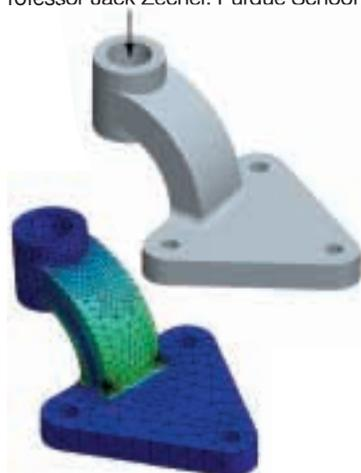
Maximum von Mises stress in a support bracket that is subjected to a 500-pound distributed vertical load
