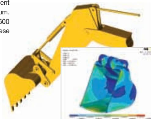
Stress and deformation of a bucket on a Caterpillar hydraulic excavator used in the modeling project
