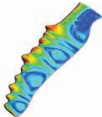
Contours of wall shear for a full-scale Reynolds number flow past a whale fin with tubercles
