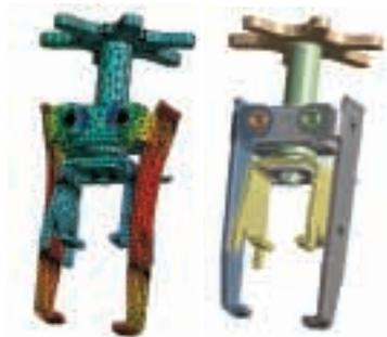
Deformation of an automotive spring compressor
